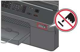
Warning—Potential Damage: Do not touch any cables, ports, any network adapter, any connector, the memory device, or the printer in the areas shown while actively printing, reading, or writing from the memory device. A loss of data can occur.
